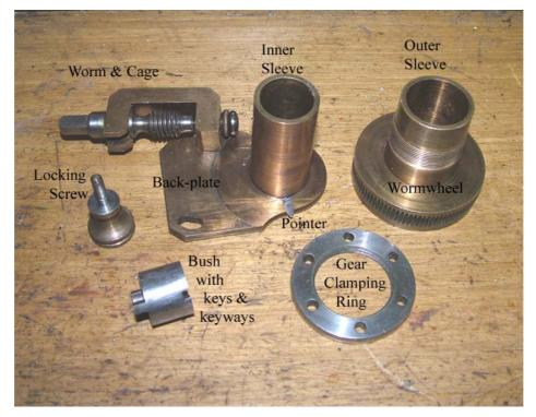
Replace the temporary screw with another having a small shoulder so that, when it is fully tightened, the cage can swing freely when the locking screw is loosened. Scribe division lines around the edge of the wormwheel, engrave numerals for every 12th division, long lines for every 6th and dots for every 4th.
