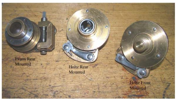
Holtz examples shown). Also the click-wheel cannot be adjusted between divisions as the worm-wheel can. The **Evans design** is superior in that it has a locking screw and a worm & wheel adjustment; this can be adjusted to any position, it can't come loose and the locking screw can't easily be broken off.
