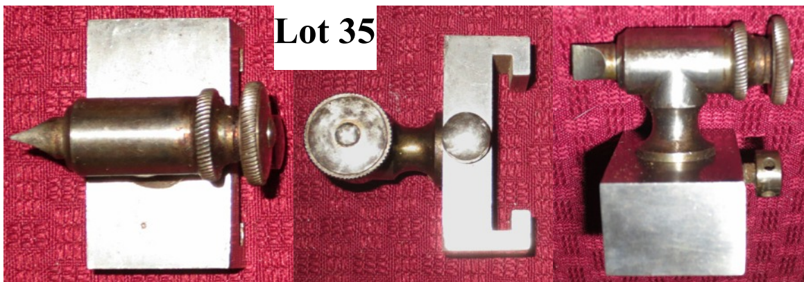
Curvilinear Rubber with adjustable depth stop. Unusual 'T' slot mount.
