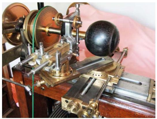
Here is a  $6\frac{1}{2}$ " height Spherical Slide-rest with the tool-slide off-set to provide extra capacity for the Horizontal Cutting Frame. This lathe has  $1\frac{1}{2}$ " raising blocks under head and tailstocks, thus raising it from 5" to  $6\frac{1}{2}$ " centre height.
