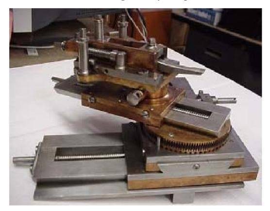
A: The tool-slide of a Spherical Slide-rest has a spigot beneath which fits into a Collar. It has a screw in the bottom for fine adjustment of the centre-height. The Tool-slide may also be rotated and clamped out of line with the rotary slide, thus allowing a Horizontal Cutting Frame held in the tool-slide to be set further back to give a larger cutting radius.
