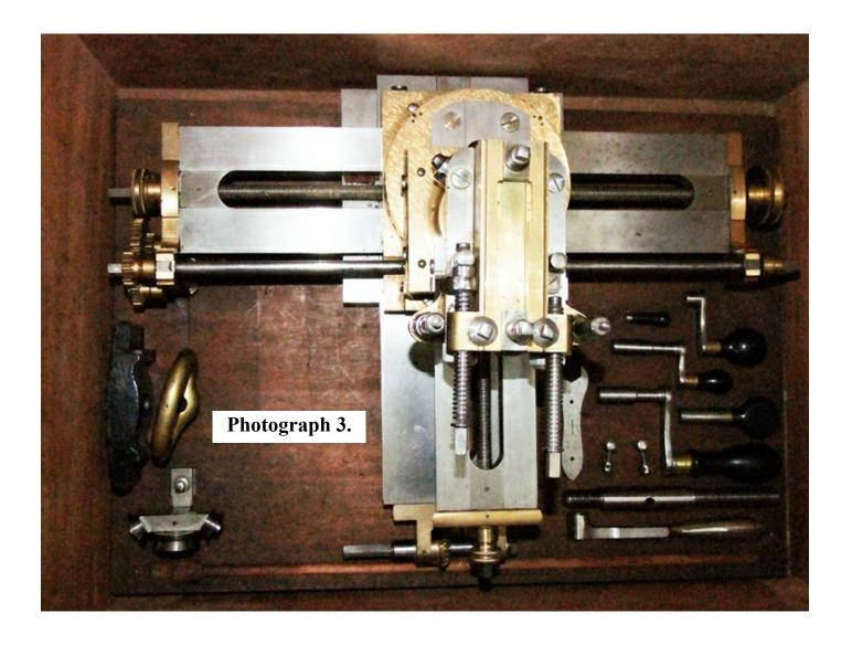
indexed for the next cut; the stop screw ensures that each cut is taken to precisely the same depth.
