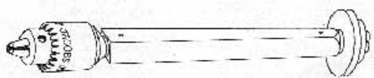
Drilling Spindle with Jacobs Chuck
