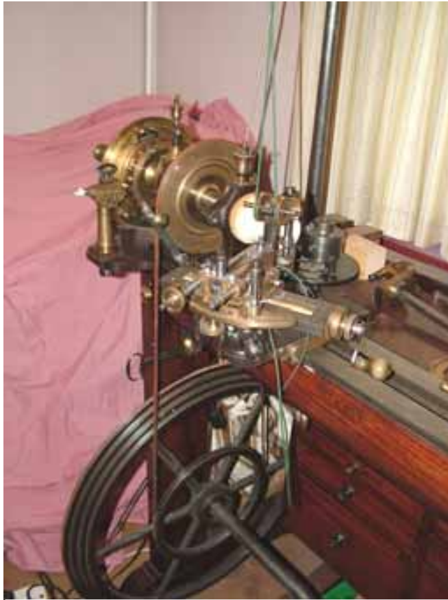
A Rose Engine and Ornamental Turning lathe by John Bower c.1840
