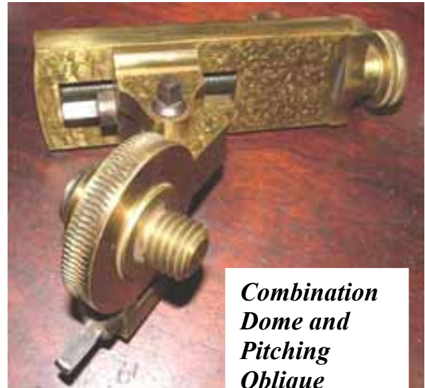
The Combination Dome/Rolling Oblique Chuck: for cutting and ornamenting round and pointed (gothic) domes.
