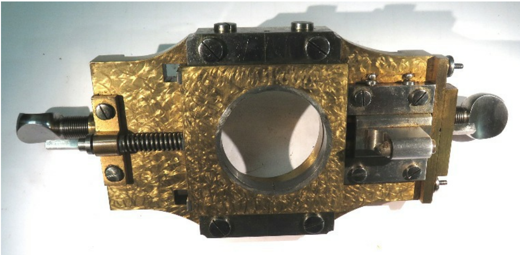
Rose Chuck, oscillating ring, pedestal for supporting the Rose chuck in front of the Spiral Dividing chuck, and set of 24 rosettes
