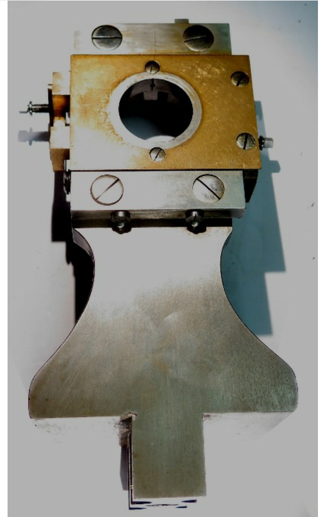
Rose Chuck, oscillating ring, pedestal for supporting the Rose chuck in front of the Spiral Dividing chuck, and set of 24 rosettes
