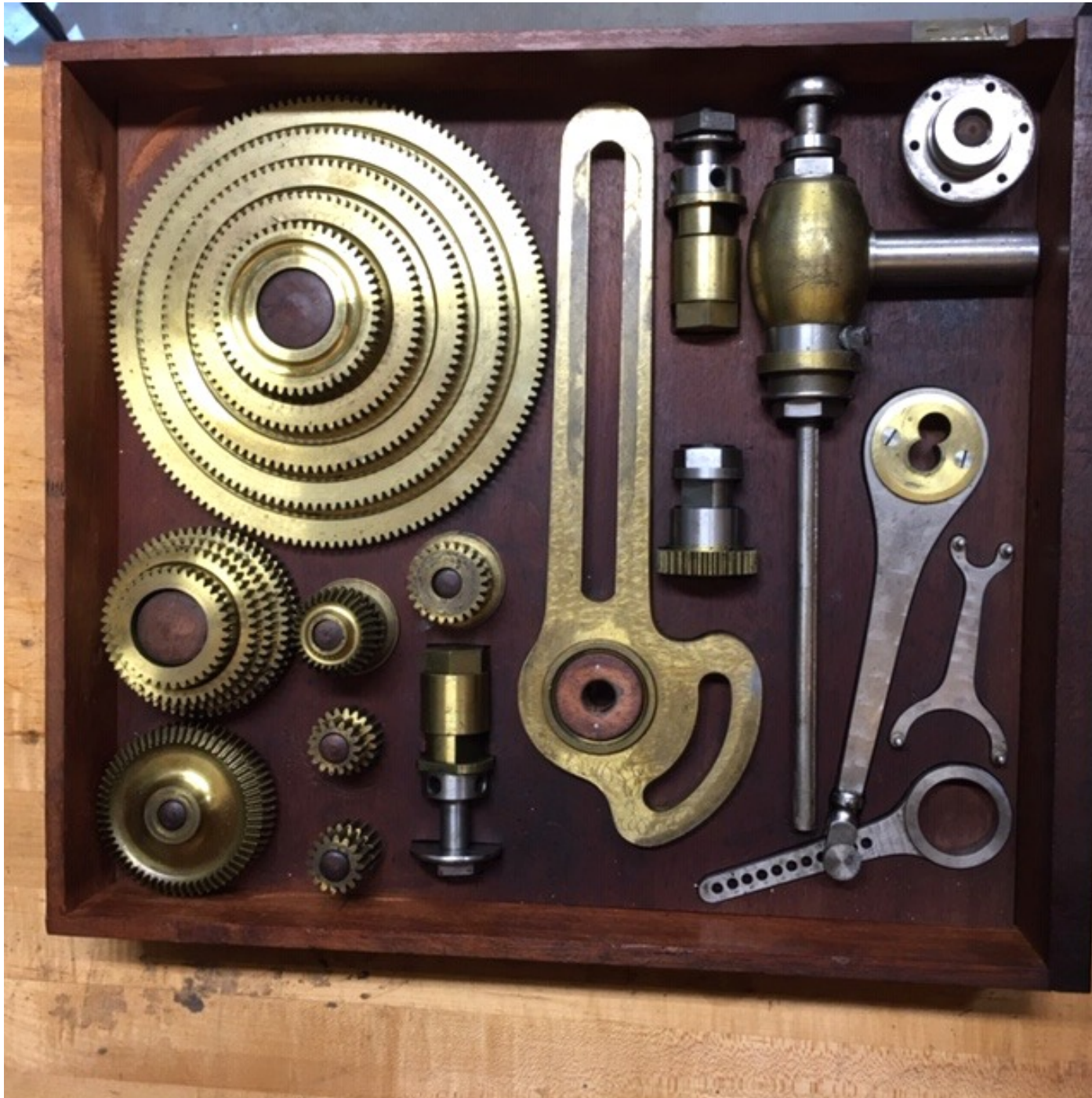
Dividing Chuck, front mounting with radial arm, reversing gear and 2 arbors; connector to slide-rest leadscrew, C spanner, set of 15 spur gears, pedestal, driving shaft, pair of bevel gears for surface spirals and Reciprocator;
