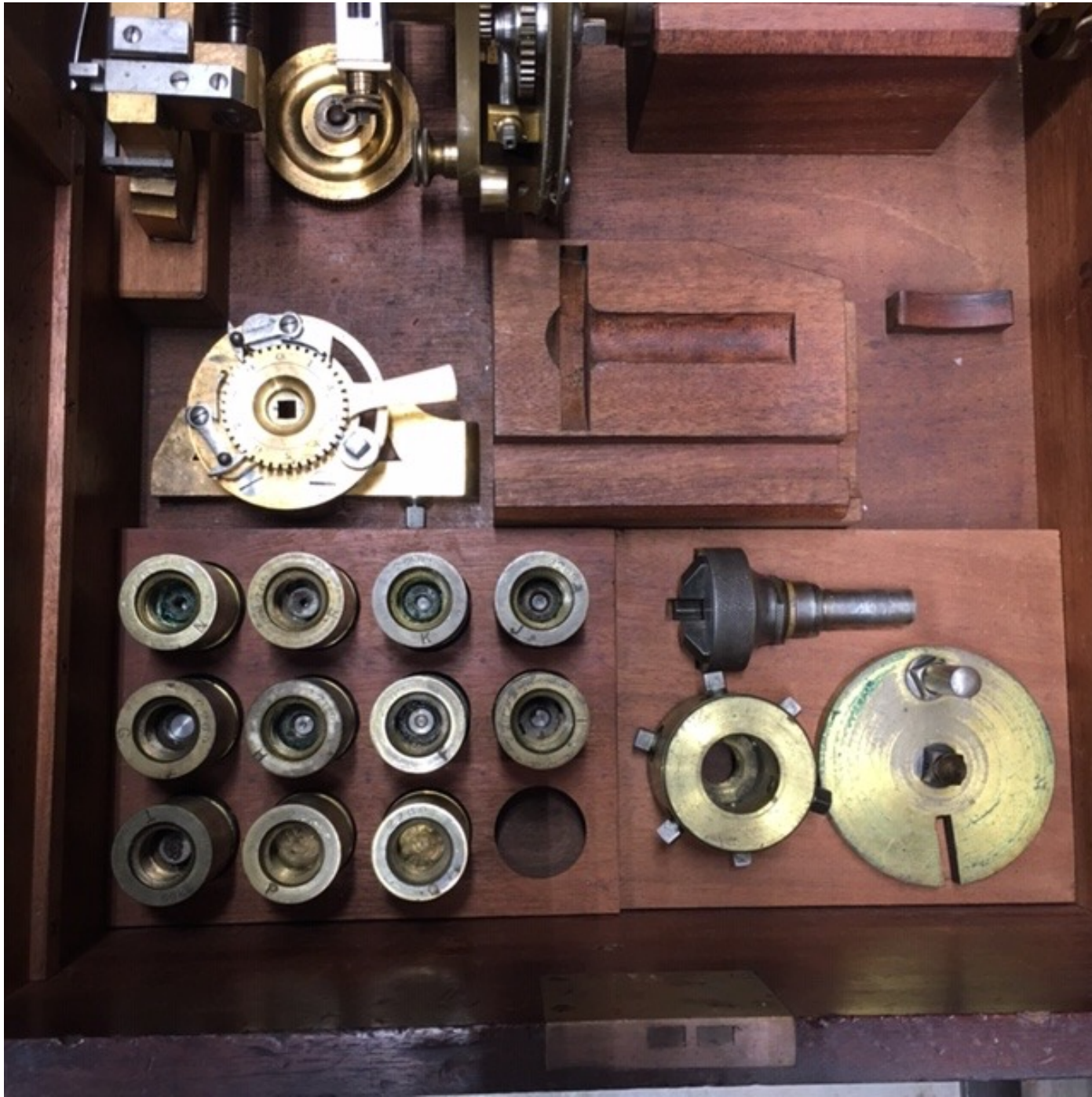
Compensating Index for the equal division of ellipses; Slow motion drive for grailing; Ratchet Counter for Slide-rest leadscrew; set of 11 male and female Drill Chucks; Hollow Screw Chuck; Driver Chuck and 3-jaw tailstock drill chuck.
