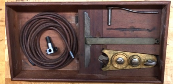
Compensating Index for the equal division of ellipses;
