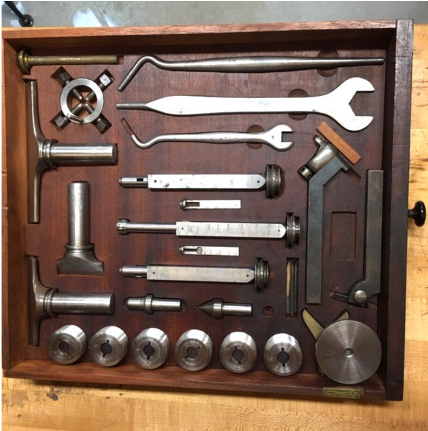
Ring Carrier 3 hand turning Tees; 2 bent bars, spanner; 2 Boring bars; Internal Cutter, Large and Small Drilling Spindles with matching honing guides; drilling pad, male and female tailstock centres and set of 6 screw-thread guides;
