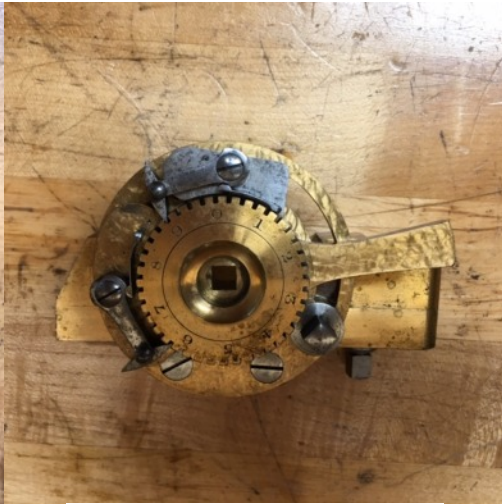
Ratchet Counter for Slide-rest leadscrew
