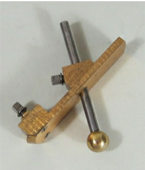
Honing Guide for round-nosed cutters.
