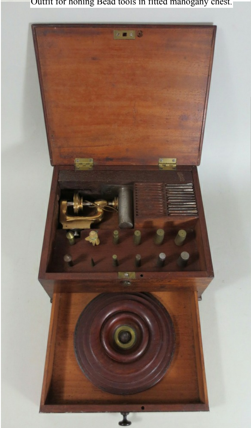
Outfit for honing Bead tools in fitted mahogany chest.
