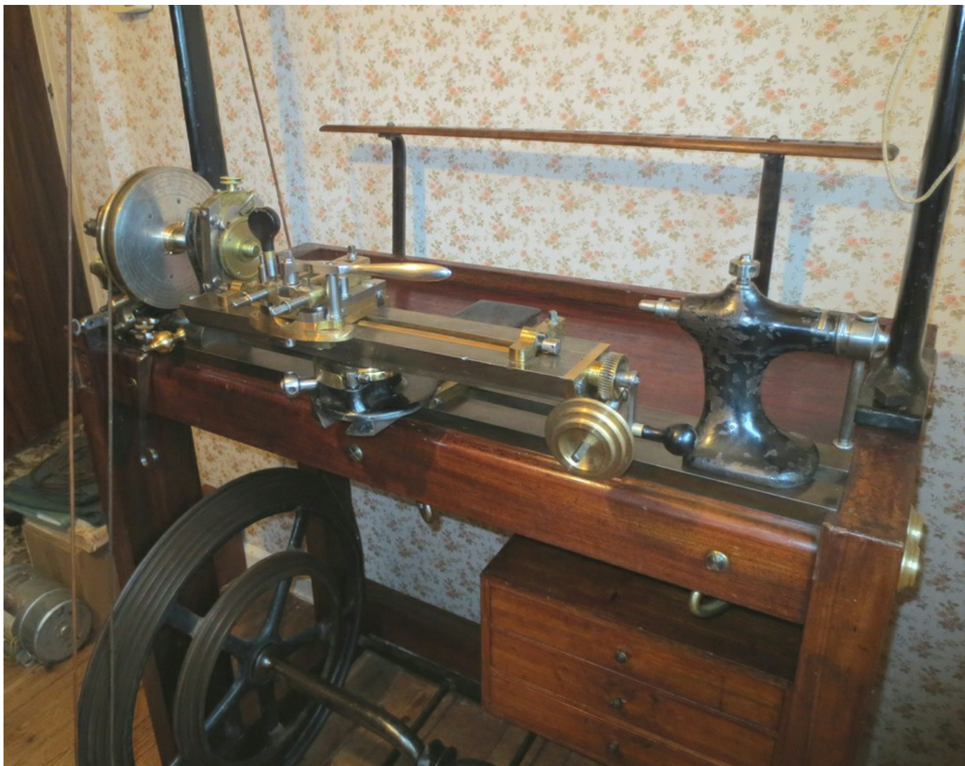
18" Ornamental Turning Slide-rest by Evans with tool-boat, steel plate, pair of tool-clamps, guide & stop screws, bridle, hand-lever, sector plate for cutting around curves, pair of fluting stops, connection to spiral apparatus with overhead drive and automatic cut-out, winch handle & key; Cradle, Clamp & Bow-nut.
