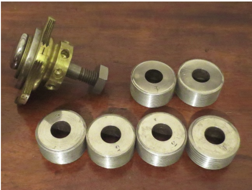
Star-nut & set of 6 Screw-thread Guides
