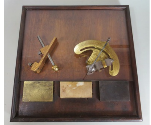
Treadle Grinding & Lapping Machine. Mahogany frame with flywheel, crank, treadle & hook; backboard poppit with cone bearing, spindle with 4 grinding wheels, water trough and tailstock; horizontal lapping machine with 3 laps; Goniostat and Honing Guide for round-nosed tools on honing board with oilstone, brass & iron laps.
