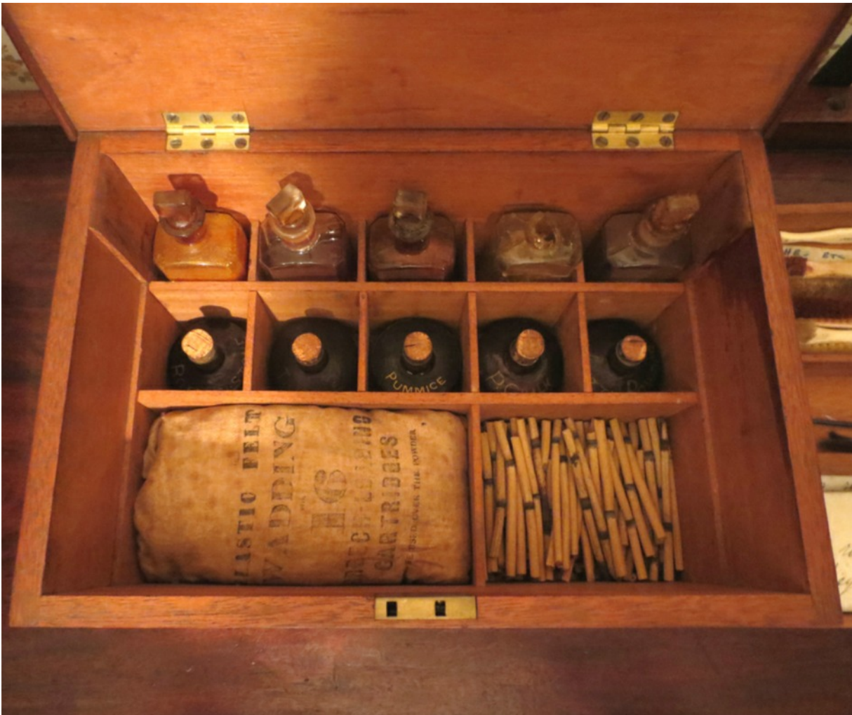
Polishing outfit with Dutch Rush, polishes & powders
