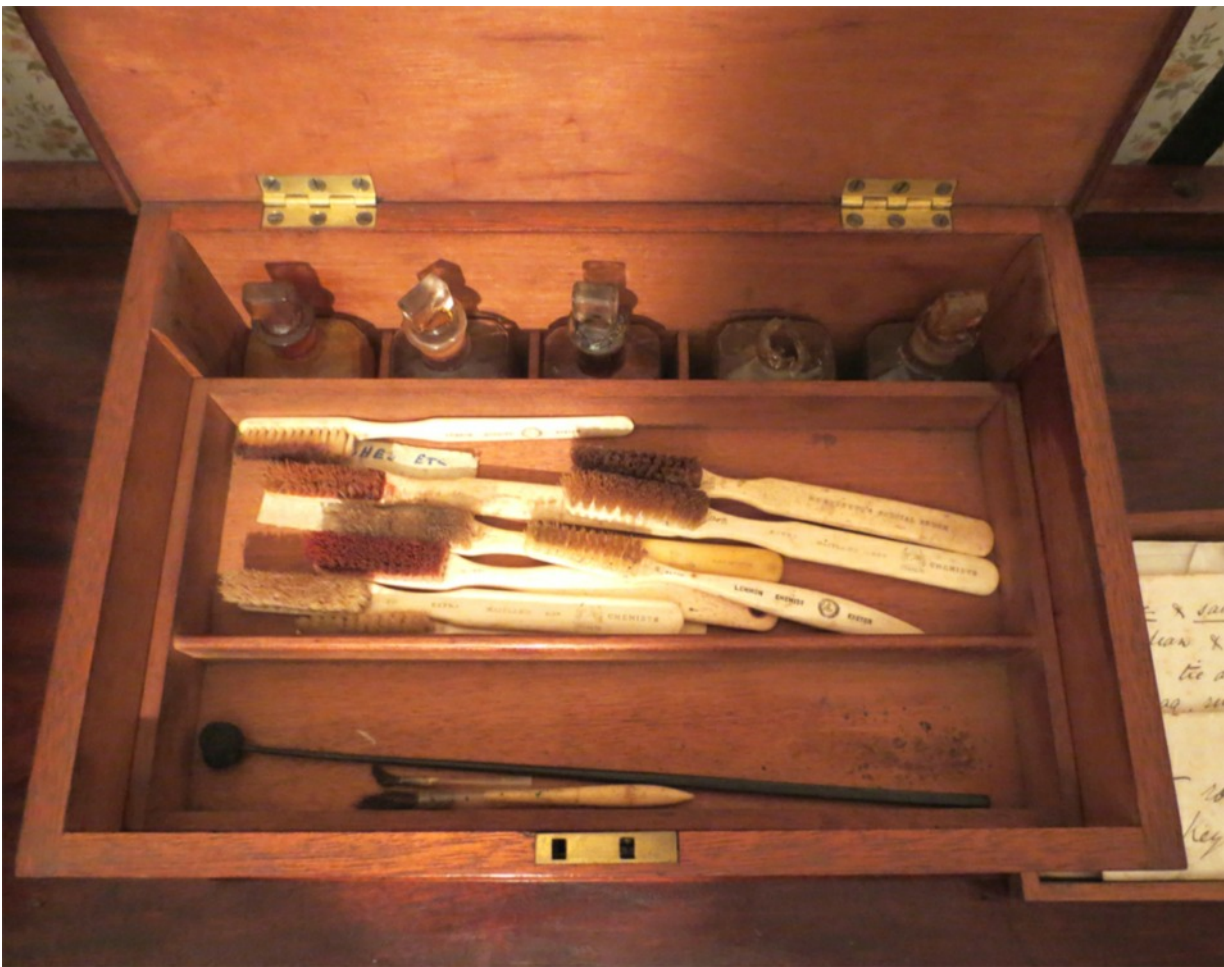
Polishing outfit with Dutch Rush, polishes & powders
