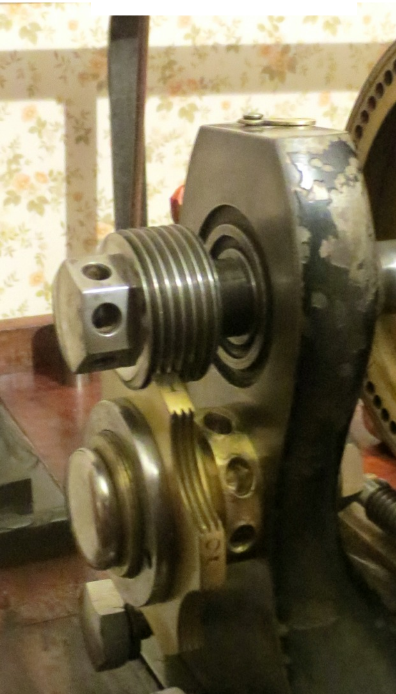
Star-nut & set of 6 Screw-thread Guides
