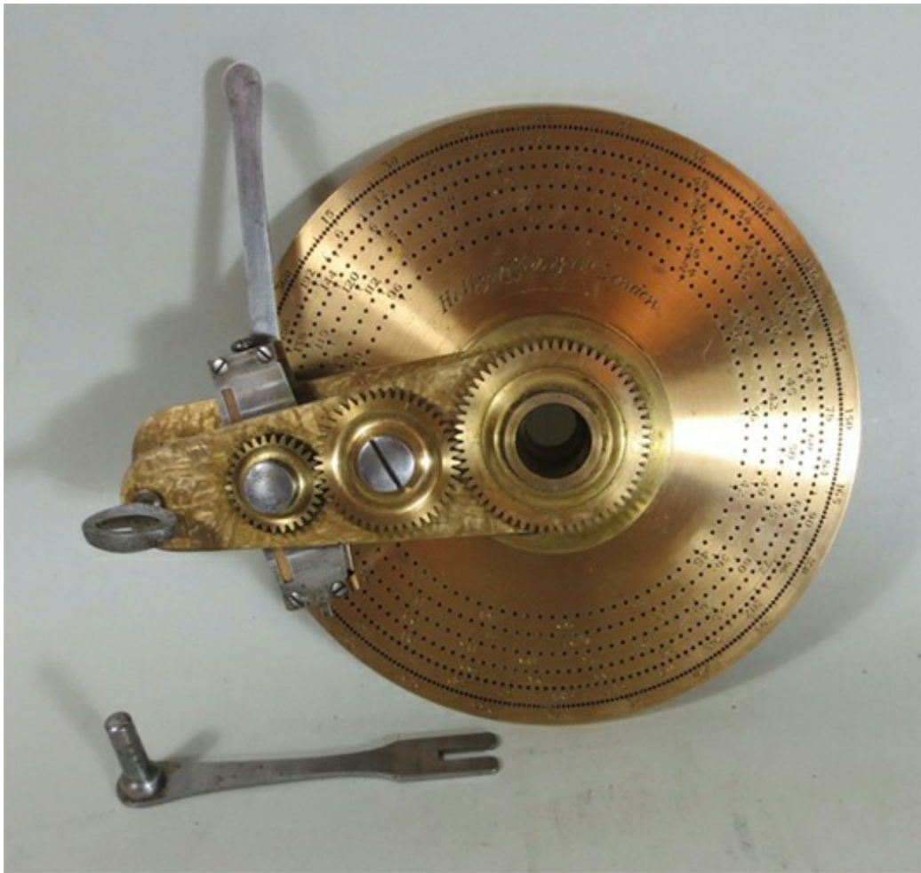
Compensating Index for equal division of the Ellipse. Designed by Evans but this one is unusual in that it was made by Holtzapffel & Co.
