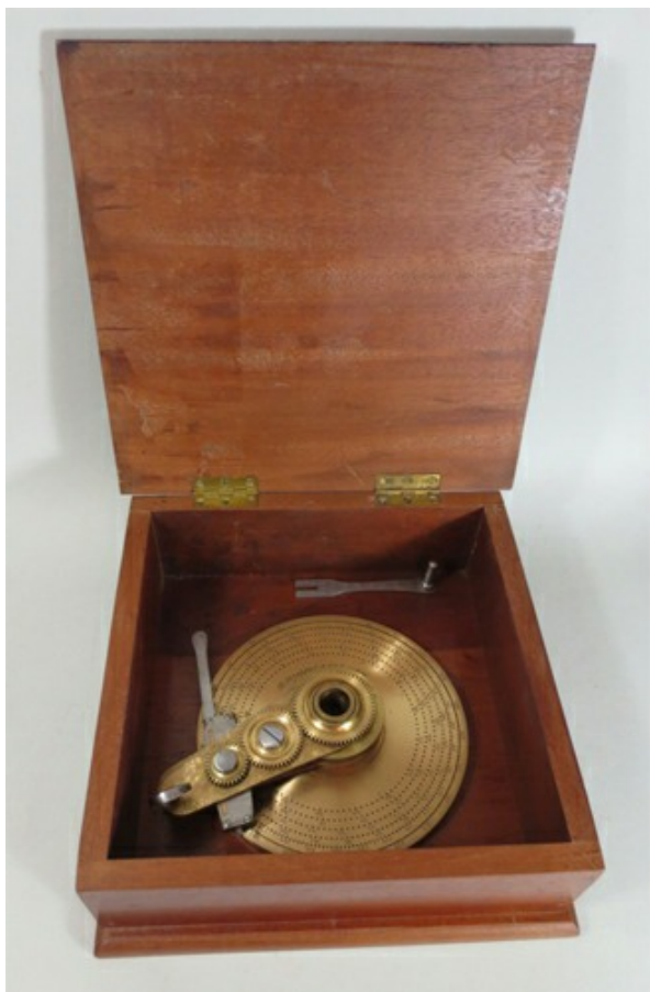
Compensating Index for equal division of the Ellipse. Designed by Evans but this one is unusual in that it was made by Holtzapffel & Co.
