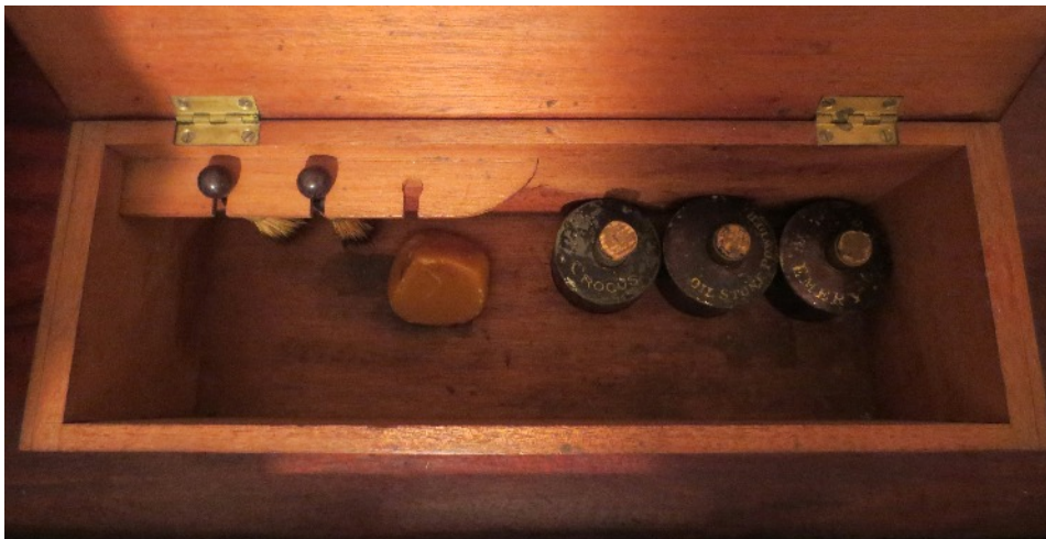
Polishing outfit with 2 (of 3) brushes & abrasive powders for honing cutters
