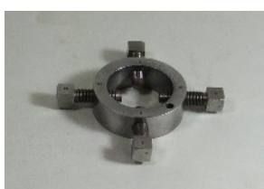
Ring Carrier & Heart Carriers for Driver Chuck
