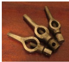
Ring Carrier & Heart Carriers for Driver Chuck
