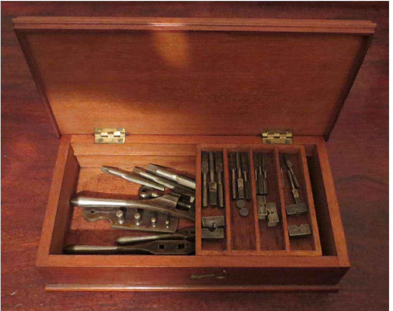
Set of Holtzapffel Taps & Dies in fitted mahogany chest.
