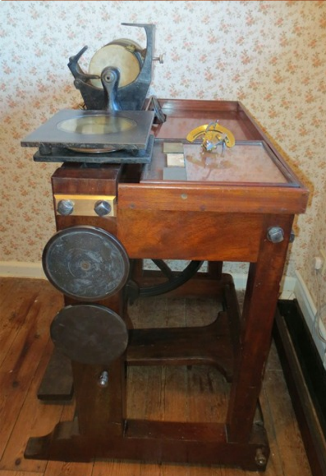
Treadle Grinding & Lapping Machine. Mahogany frame with flywheel, crank, treadle & hook; backboard poppit with cone bearing, spindle with 4 grinding wheels, water trough and tailstock; horizontal lapping machine with 3 laps; Goniostat and Honing Guide for round-nosed tools on honing board with oilstone, brass & iron laps.
