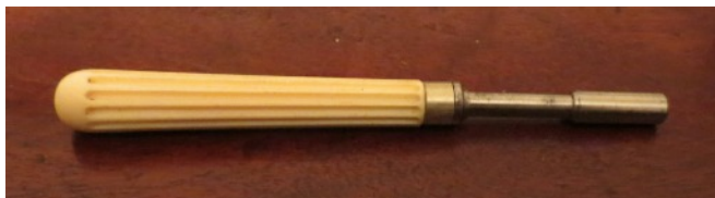
Compensating Index for equal division of the Ellipse. Designed by Evans but this one is unusual in that it was made by Holtzapffel & Co.
