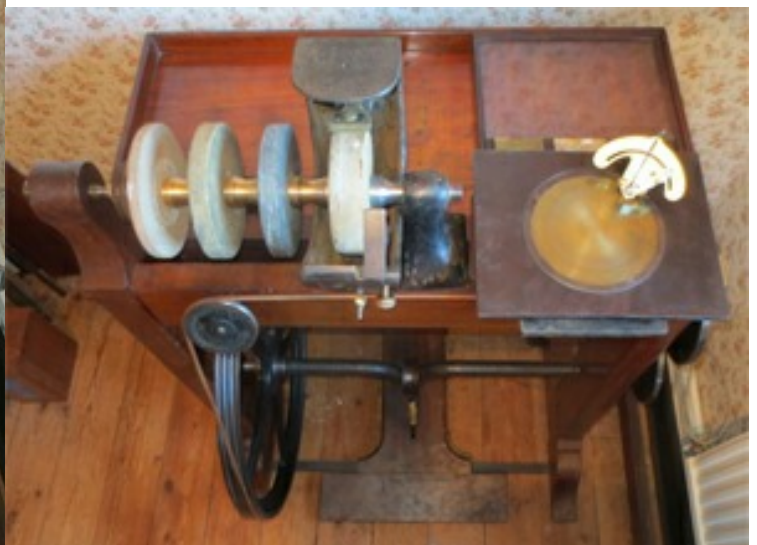
Treadle Grinding & Lapping Machine. Mahogany frame with flywheel, crank, treadle & hook; backboard poppit with cone bearing, spindle with 4 grinding wheels, water trough and tailstock; horizontal lapping machine with 3 laps; Goniostat and Honing Guide for round-nosed tools on honing board with oilstone, brass & iron laps.
