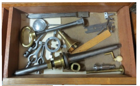
Drawer 3 containing Saw blade and spindle; bell punch (2); Ring Carrier & Heart Carrier (3) for Driver Chuck; Oilcan and sundry items.
