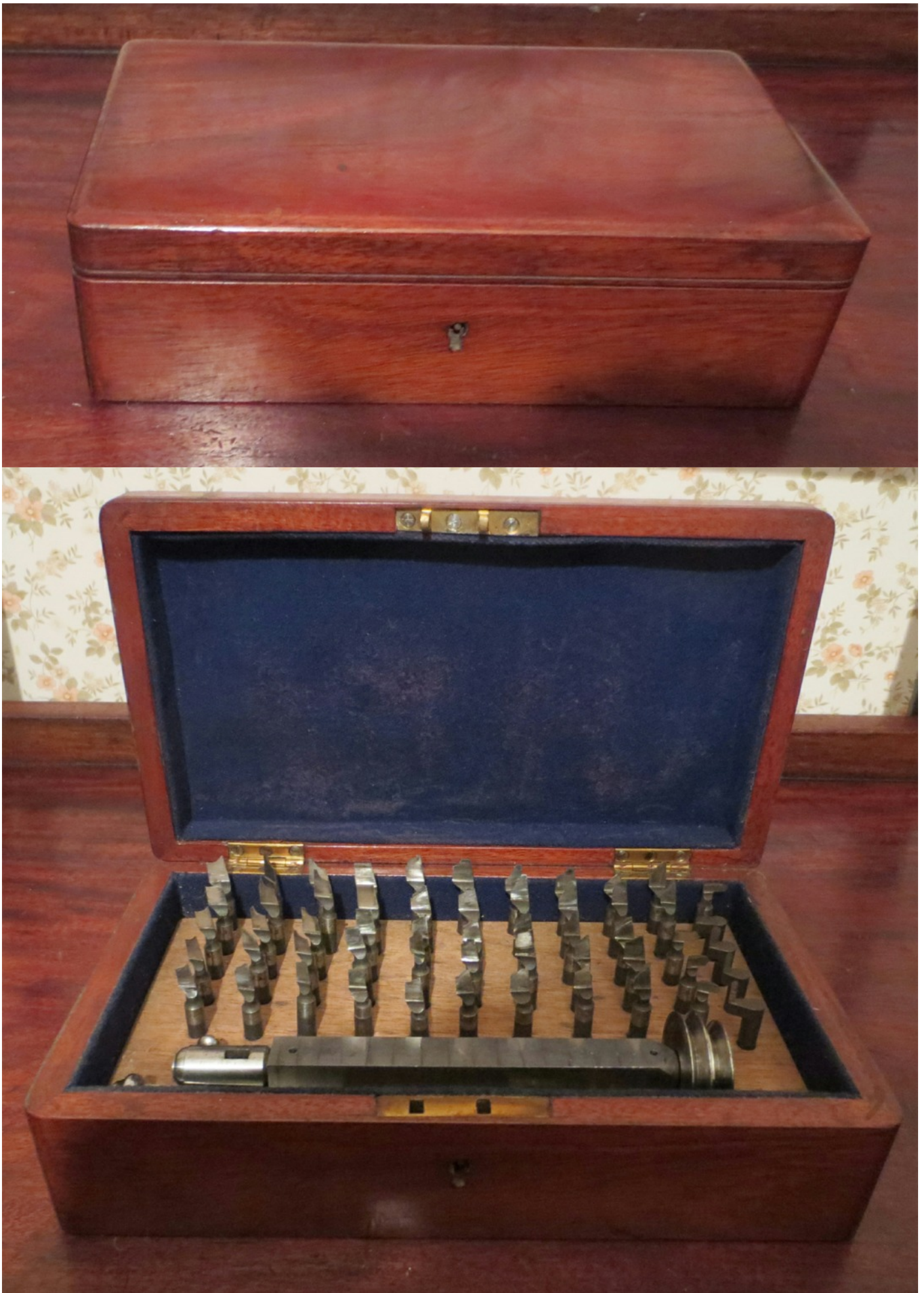
Drilling Spindle with set of 55 drills & honing guide in fitted mahogany chest
