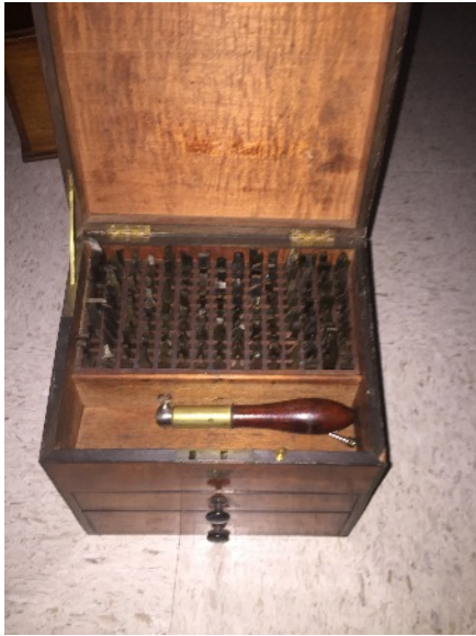
Slope-top Mahogany Chest with 168 slide-rest cutters, 144 ECF cutters, 36 small UCF cutters, 72 small drills with matching Drill Spindle (on page 7) and a Pad Handle,
