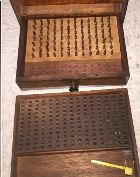
Slope-top Mahogany Chest with 168 slide-rest cutters, 144 ECF cutters, 36 small UCF cutters, 72 small drills with matching Drill Spindle (on page 7) and a Pad Handle,
