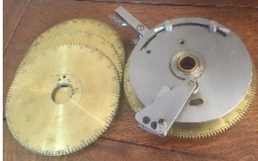
sets of 6 Holtzapffel & 6 Whitworth screw guides and star-nuts for thread cutting
