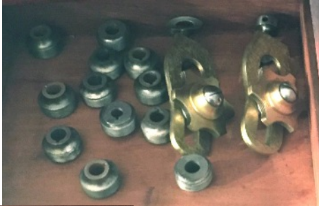
Ashton's Automatic Counting Index with 4 division plates;
