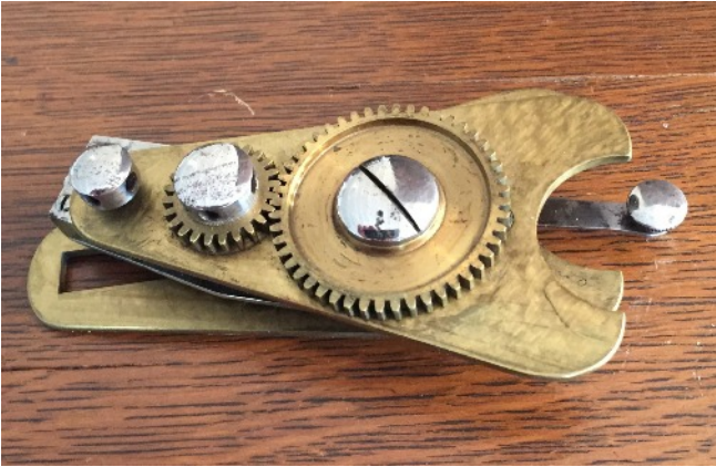
Compensating Index for equal division of the ellipse
