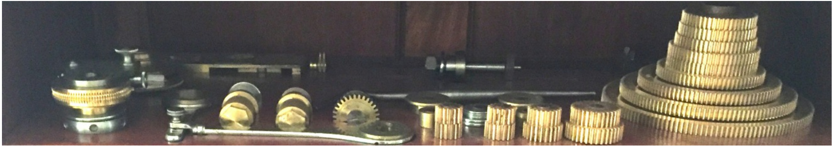
Dividing Chuck & Spiral Apparatus (rear-mounting) with gears & arbors,
