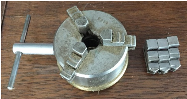
3-jaw S.C. chuck with inside & outside jaws (modern),
