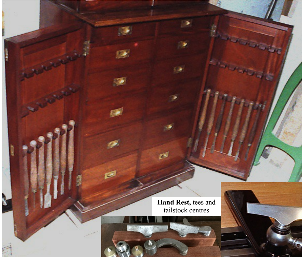
Large Mahogany Tool Cabinet with upper tier of shelves enclosed by glazed doors and lower tier of 12 drawers enclosed by panelled doors fitted with 14 long-handles and 21 of 24 short-handled turning tools the cabinet (see also page 9).
