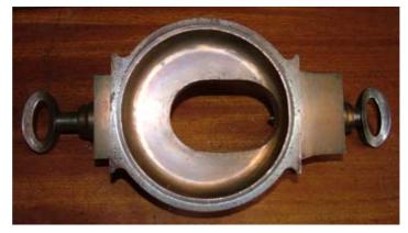
steel Sliding Block on it. Top quality Trade Rose Engines have chucks made like this and the diameter of their ring ranges from around 6" to as much as 10".
