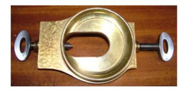
mandrel by up to 1" of eccentricity; i.e. an ellipse may be cut with a maximum difference between the minor and major axes of 2". So, the answer is - make the ring as large as you can; a ring of 4" outer diameter is adequate but a larger ring can give a greater range of movement.
