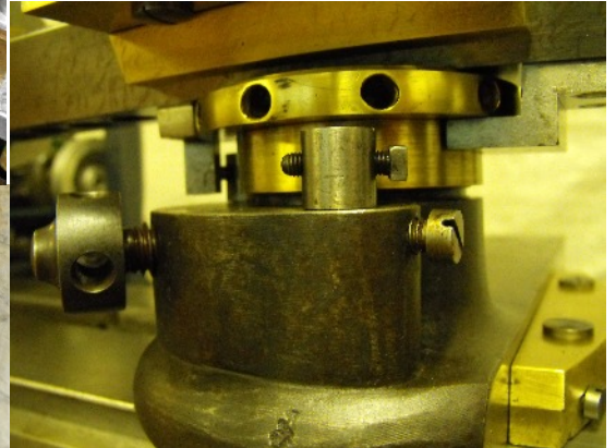
Ornamental Slide- rest with height adjustment
