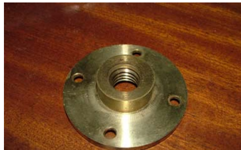
Back-plate to be inserted and screwed onto wooden pad
