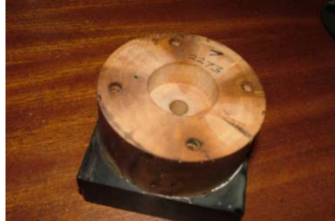
Wooden pad glued to workpiece
