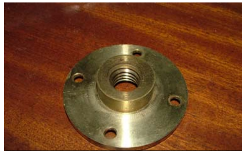
Back-plate to be inserted and screwed onto wooden pad
