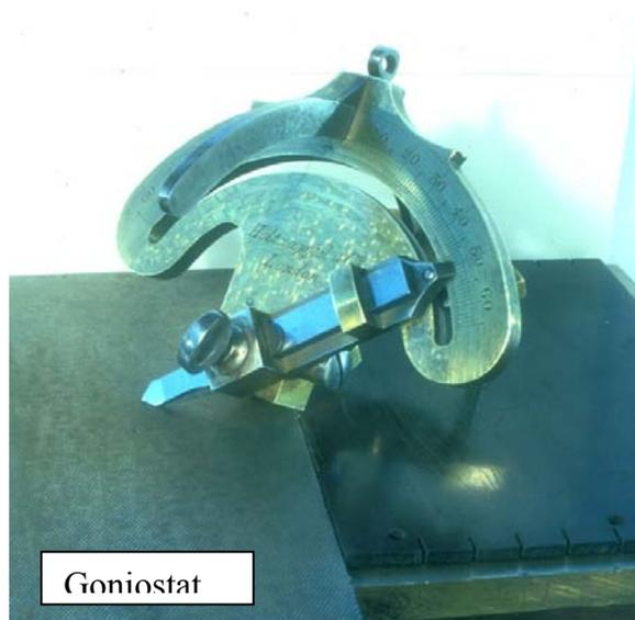
The best results come from using diamond paste (diamond dust mixed with grease) on a flat ceramic lap (ceramic laps are expensive so you might try a very flat ceramic wall tile); any softer surface will soon become abraded and no longer flat. I start with a coarse diamond impregnated lap, then a fine one, then the ceramic lap, using a range
