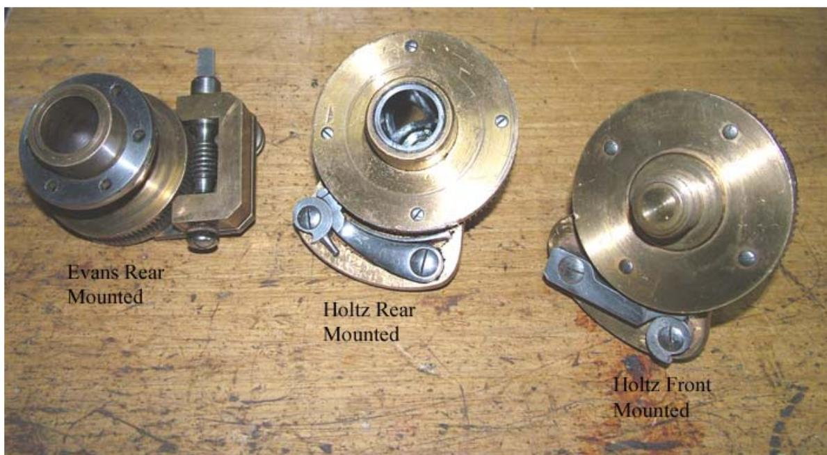
Holtz examples shown). Also the click-wheel cannot be adjusted between divisions as the worm-wheel can. The **Evans design** is superior in that it has a locking screw and a worm & wheel adjustment; this can be adjusted to any position, it can't come loose and the locking screw can't easily be broken off.
