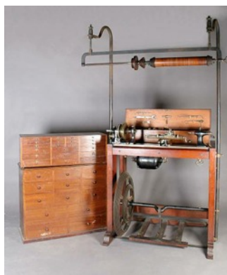
Top of the range Ornamental Turning Lathe by Holtzapffel refurbished 1893
